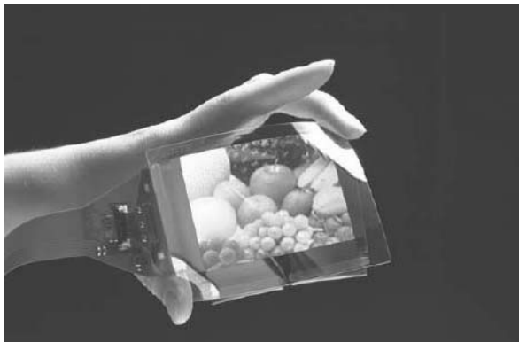
Figure 8.17. OLED 3'' passive display on a PET plastic substrate (source: Pioneer 2002) (see color plate section)
