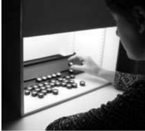
Figure 7.21. Experimental handling of colored objects in a cabin exposed to LEDs
