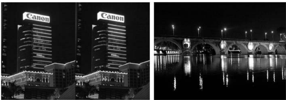
Figure 1.12. Left: LED illumination of the Canon tower in Kowloon (Hong Kong) 14 lines with 30 LEDs per line. Each chip consumes 6 W and includes six junctions (2 red, 2 green and 2 blue), for a total power of 12.5 kWh per night [LED 07]; right: arches of the Pont Neuf bridge in Toulouse have been illuminated since November 2007 with a dynamic LED lighting (total power 1 kW)(see color plate section)
